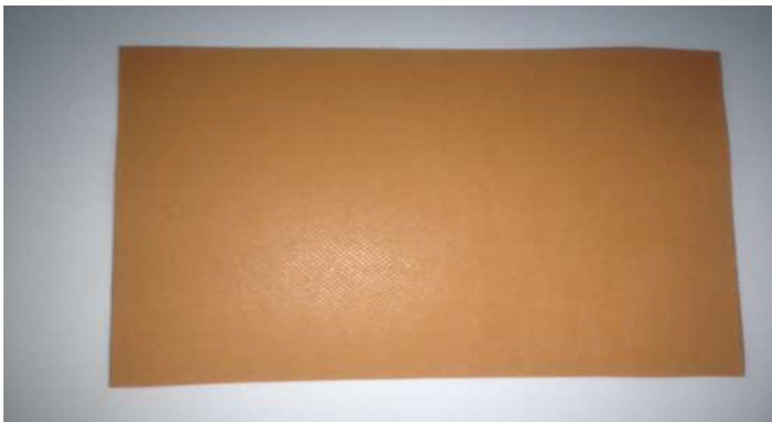
Figure 2. Polypropylene base cloth after E883D Termite Barrier coating layers
